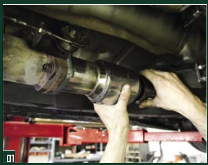
1) The MetalCat comes with reducers, but as this one had 2.5in reducers, Rocco's cut them off at the right point to weld on 3in pipes
